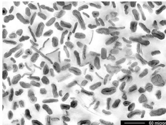
**Fig. 4** Cross-section of a natural bamboo fiber
