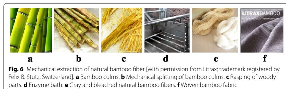
**Fig. 6** Mechanical extraction of natural bamboo fiber [with permission from Litrax; trademark registered by Felix B. Stutz, Switzerland]. **a** Bamboo culms. **b** Mechanical splitting of bamboo culms. **c** Rasping of woody parts. **d** Enzyme bath. **e** Gray and bleached natural bamboo fibers. **f** Woven bamboo fabric
