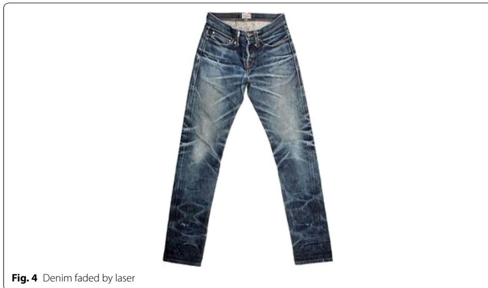
make engravings on them. Laser engraving is used to engrave the printing screens, for hollowing, for creating pattern buttons, to engrave leather, denim etc. (Fig. 5). Pictures, flower patterns and even personalized signatures can be engraved on leather shoes, leather bag, wallet, leather belt, leather sofa and leather clothes, greatly increasing the added value of products. In addition laser engraving is used to create embroidered
