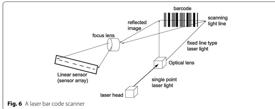
**Fig. 6** A laser bar code scanner
