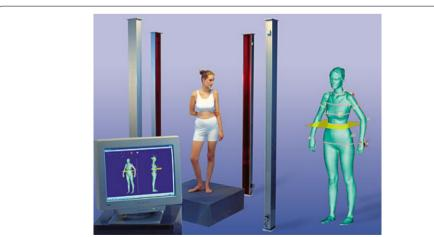
Fig. 3 3D body scanning by Laser scanner
