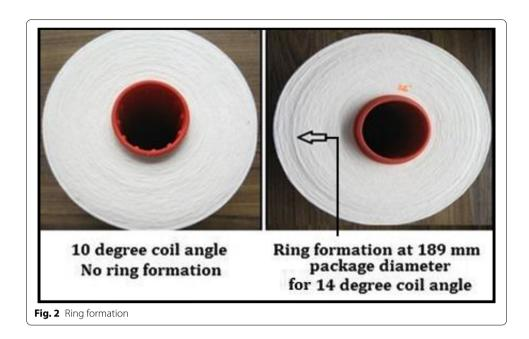
The table developed was transferred to Peass UFlex rewinding machine through software and winding trials were conducted and packages for the entire range of coil angles were produced to confirm winding trial in continuous run.
