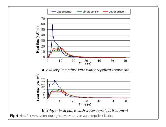
soil from the fabric (Kissa 1981). This process of drawing in moisture may be the reason for absorbing more energy. As the twill woven fabrics are heavier and thicker than the plain woven fabrics it is possible that this added effect of absorbing more hot liquid made the twill fabrics store more energy than the plain fabrics.
