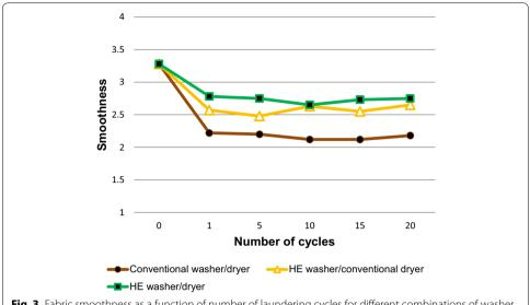
**Fig. 3** Fabric smoothness as a function of number of laundering cycles for different combinations of washer and dryer used
