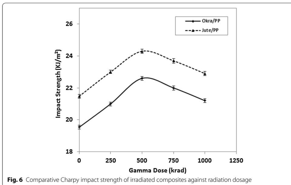
23% development in BS, 48% increase in BM and 13% increment in IS was found compared to the non-irradiated specimen.
