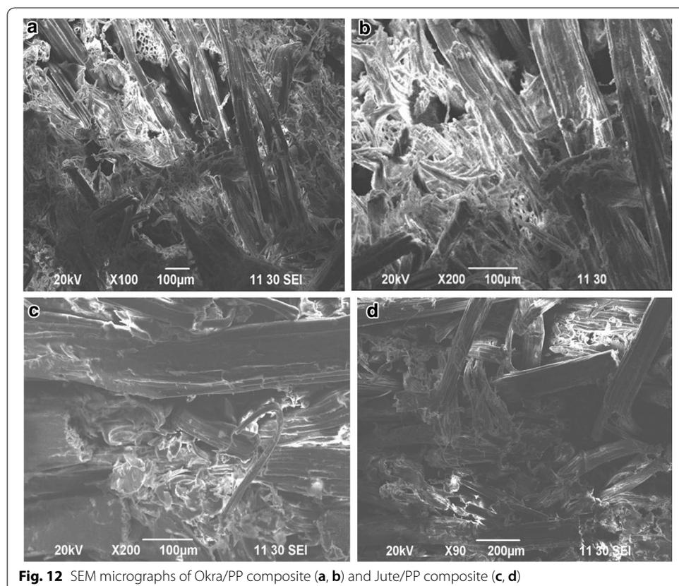
**Fig. 12** SEM micrographs of Okra/PP composite (a, b) and Jute/PP composite (c, d)
