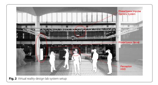
and determines their location in the courtyard. The LED markers are attached to headmounted displays (HMDs). Each user wears a HMD with LED markers that emit unique light signals visible to the camera system. The camera server, the last part of the tracking system, process the data collected from each camera module to locate the actual positions of the participants within a 1-mm accuracy.
