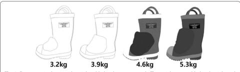
**Fig. 1** Fire protective boots with weight added in the present study. The weight were added to the right and left boot evenly. The 3.2, 3.9, 4.6 and 5.3 kg demonstrate the total sum of right and left boot mass
