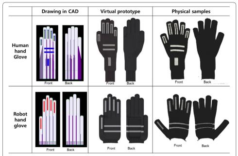
**Fig. 7** Glove design with sensor units, the simulated virtual front and back gloves, and knitted prototypes for the human hand and robotic hand
