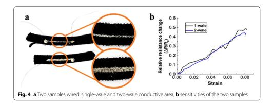
sensors with conductive areas with one- and two-wale rectangular shapes. Since their initial resistances were different, further experiments were conducted to determine which one was more suitable for the glove sensors: producibility and sensitivity.
