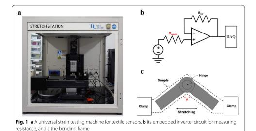
to and output from the op-amp in the circuit, which is depicted as a triangular shape in Fig. 1b. Then, the measured data were collected by the data acquisition system (DAQ).
