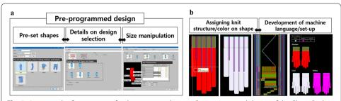
**Fig. 3** Automated software system for design manipulation. **a** Pre-programmed shapes of the Glove, Socks, KnitCap, Bottom, and Tubular shape, including design options and hand measurements, and **b** assignment of knit structures and patterns with the development of machine language for knitting
