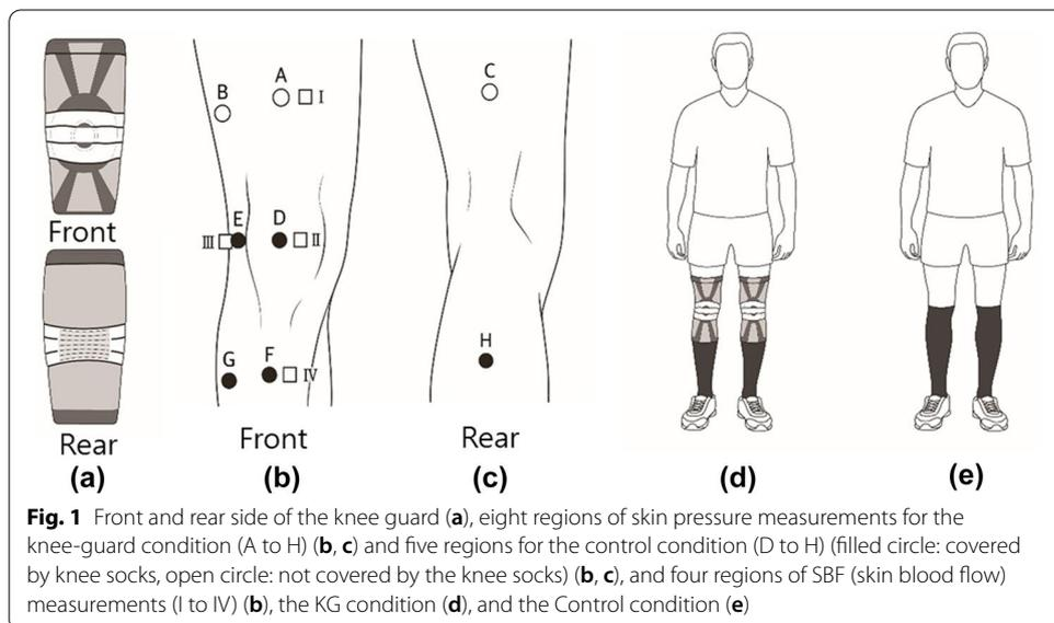
**Fig. 1** Front and rear side of the knee guard (a), eight regions of skin pressure measurements for the knee-guard condition (A to H) (b, c) and five regions for the control condition (D to H) (filled circle: covered by knee socks, open circle: not covered by the knee socks) (b, c), and four regions of SBF (skin blood flow) measurements (I to IV) (b), the KG condition (d), and the Control condition (e)
