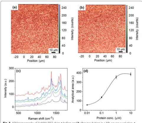
**Fig. 3** AFM tomography of AgNWs/PET chips **a** before and **b** after incubation in a Mb aqueous solution. **c**, **d** SERS detection with AgNWs/PET chips. **c** SERS spectra of Mb solutions with concentrations ranging from  $10^{-8}$  M to  $10^{-5}$  M (black, naked chip; violet,  $10^{-8}$  M; green,  $10^{-7}$  M; blue,  $10^{-6}$  M; red,  $10^{-5}$  M). **d** Correlation between the 756 cm<sup>-1</sup> band area and protein concentration (error bars represent the standard deviation)
