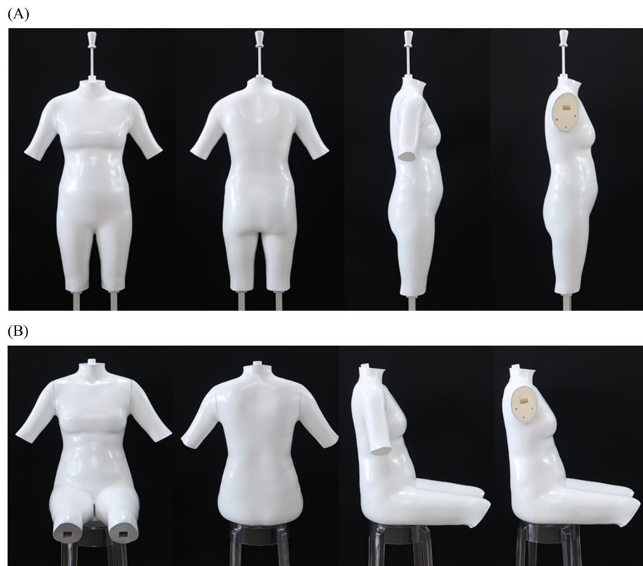
Fig. 5 3D printed full-size dress form in a standing posture (A) and a sitting posture (B)
