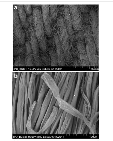
Figure 1 Scanning electron micrograph of denim garment: (a) untreated denim garment and (b) untreated denim garment (magnified).
