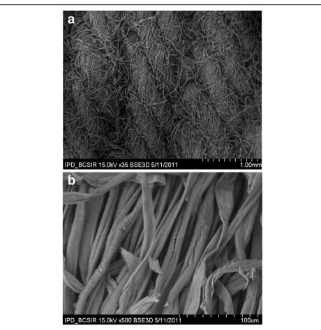
Figure 2 Scanning electron micrograph of denim garment: (a) after enzyme treatment and (b) after enzyme treatment (magnified).
