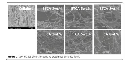
cross-linked cellulose fibers were similar to the pristine cellulose fiber regardless of the cross-linking agent types. As the concentration of the cross-linking agent increased over 5 wt%, the membrane-like shape started to appear. The further increase of the agent concentration resulted in film-like web morphology. This morphology change was similarly was observed in other researches (Chen et al. 2012; Liu et al. 2007).
