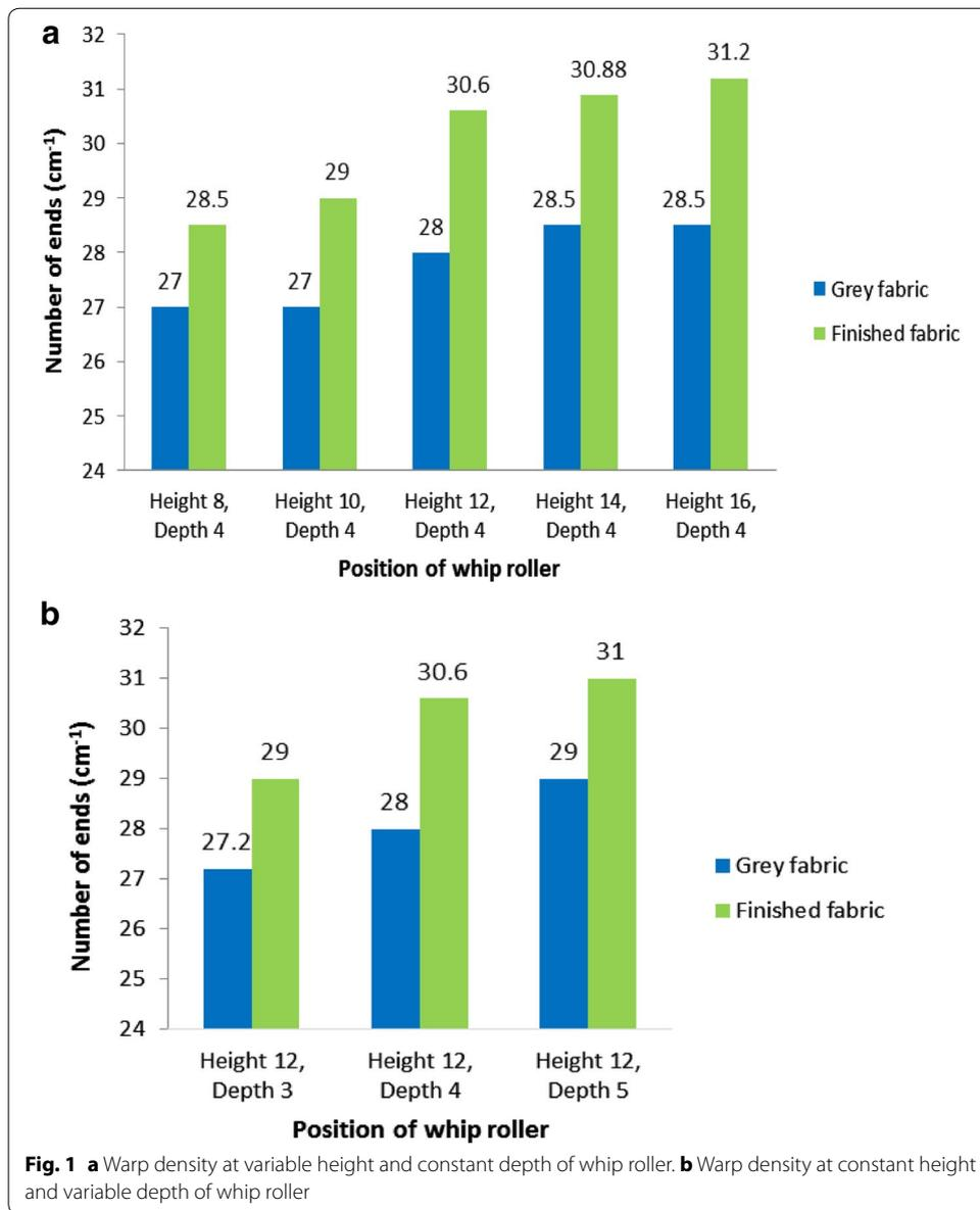
The above graph showed that with increasing the height of backrest roller's position at constant depth, warp density of grey and finished fabric also increased but slightly. Comparing to grey fabric, finished fabric had greater change in this property due to being passed through a number of finishing treatments. When backrest roller's depth decreased at constant height same results were found.
