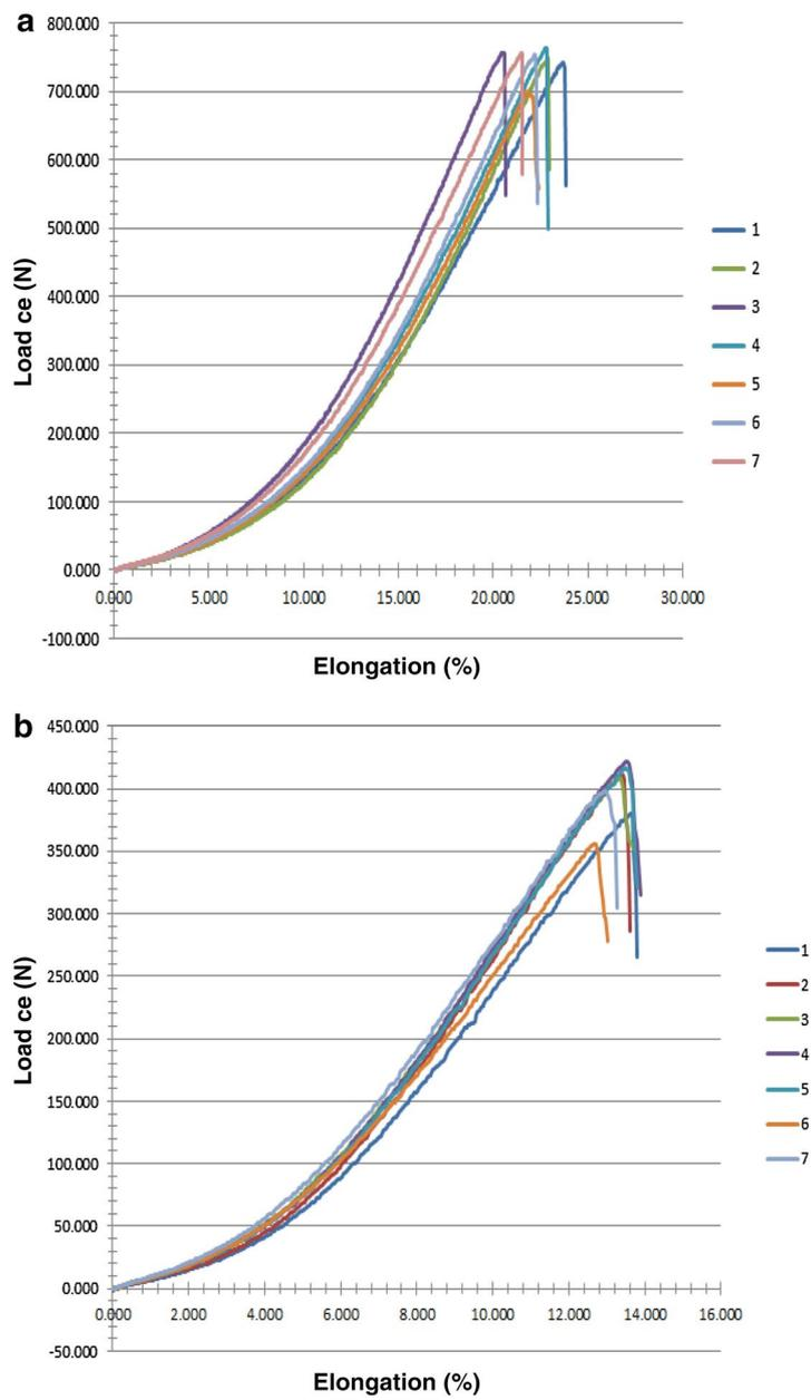
**Fig. 7** Load-elongation curve of grey fabric both in warp **(a)** and weft **(b)** direction
