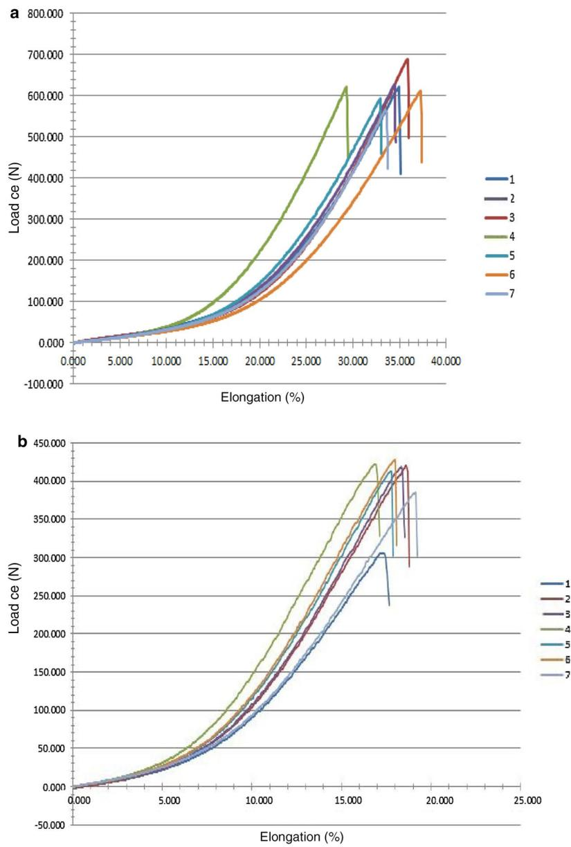
**Fig. 8** Load-elongation curve of finished fabric both in warp (a) and weft (b) direction
