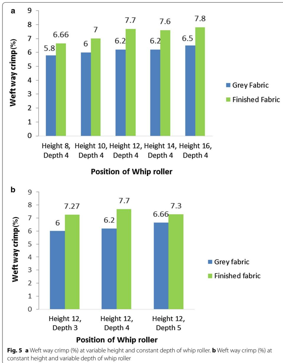
But in Fig. 11b a different trend was observed. When depth of whip roller’s position was decreased at constant height, shrinkage decreased in both state because tension of warp yarns was gradually decreased at long shed area. It was also seen in both figures that shrinkage was lower in finished fabric than grey fabric because of finishing treatment on denim.
