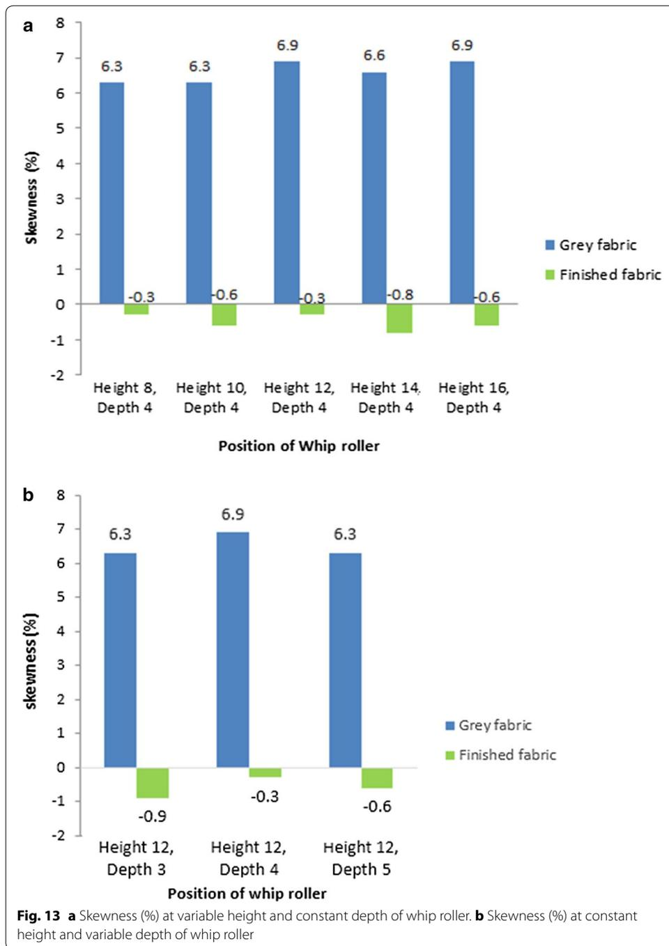
due to different finishing treatment. Generally whip roller setting is kept unchanged in different woven fabric production. But it directly affects EPcm and PPcm which change the cover factor of fabric. Moreover, the research result shows that it also deviates different physical properties of fabric. So if this position is optimized, fabric properties can be enriched as well as faults can be minimized.
