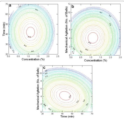
Fig. 2 a K/S vs concentration and time for acid cellulase on sulphur dyed denim. **b** K/S vs concentration and mechanical agitation for acid cellulase on sulphur dyed denim. **c** K/S vs time, mechanical agitation for acid cellulase on sulphur dyed denim
