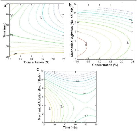
**Fig. 3 a** K/S vs concentration and time for neutral cellulase on indigo dyed denim. **b** K/S vs concentration and mechanical agitation for neutral cellulase on indigo dyed denim. **c** K/S value vs time and mechanical agitation for neutral cellulase on indigo dyed denim
