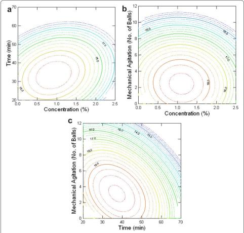
**Fig. 4** a K/S value vs concentration and time for neutral cellulase on sulphur dyed denim. **b** K/S value vs concentration and mechanical agitation for neutral cellulase on sulphur dyed denim. **c** K/S value vs time and mechanical agitation for neutral cellulase on sulphur dyed denim
