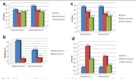
**Fig. 5** a Colour strength (K/S value) on enzyme washing. **b** Weight loss (%) on enzyme washing. **c** Colour strength (K/S values) of sulphur dyed denim on Denimax treatment. **d** Back-staining levels on white cotton lining
