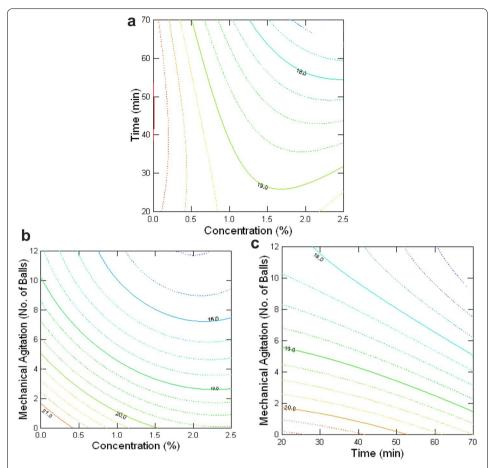
**Fig. 1 a** K/S vs concentration and time for acid cellulase on indigo dyed denim. **b** K/S vs concentration and mechanical agitation for acid cellulase on indigo dyed denim. **c** K/S vs time and mechanical agitation for acid cellulase on indigo dyed denim
