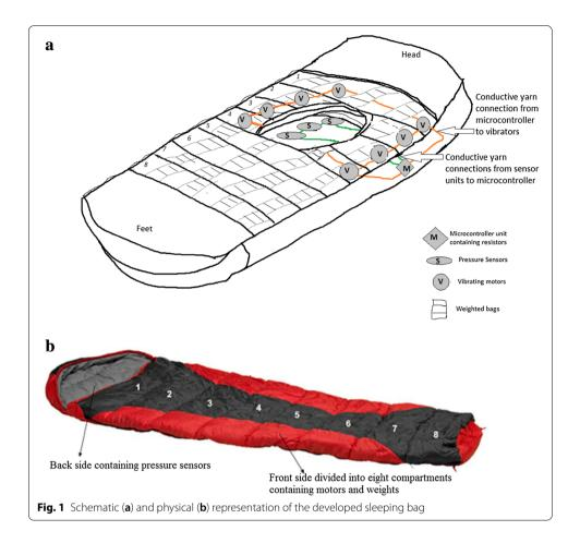
front part provide continuous deep pressure stimuli and can be adjusted by removing any number of weighted bags according to wearer's comfort level.
