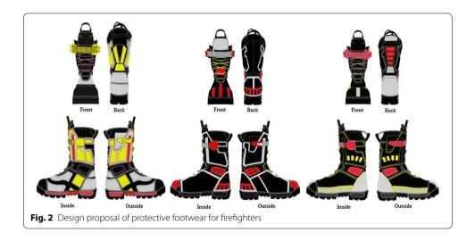
Figures 3, 4 and 5 show the pattern design plan of the three improved designs of protective footwear for firefighters, and the test products I, II, and III. The material used for the test products were synthetic leather and rubber. The opening that uses laces and buckles make it easy to wear and take off fast. Different size adjustments can be made to fit different body types, and there is closer contact at the ankles. All test prototypes, the size is 265 cm and the weight is about 1.3 kg.
