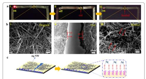
**Fig. 4 a** Photographs of an LED integrated with Ag nanowires/PnBA-g-PAN elastomer for self-healing tests. **b** SEM images of Ag nanowire/PnBA-g-PAN composite elastomer conductor: (i) original one, (ii) after being cut, and (iii) after healing. **c** The healing mechanism of composite elastomer by dynamic interactions
