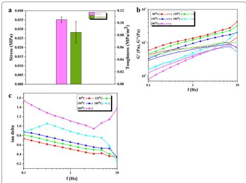
**Fig. 3** a stress at break and toughness of PnBA-g-PAN; **b** Storage modulus (G', solid symbols) and loss modulus (G', hollow symbols) for PnBA-g-PAN graft copolymer elastomer as a function of frequency at different temperatures; **c** dissipation factor (tan  $\delta$ ) of PnBA-g-PAN graft copolymer elastomer as a function of frequency at different temperatures
